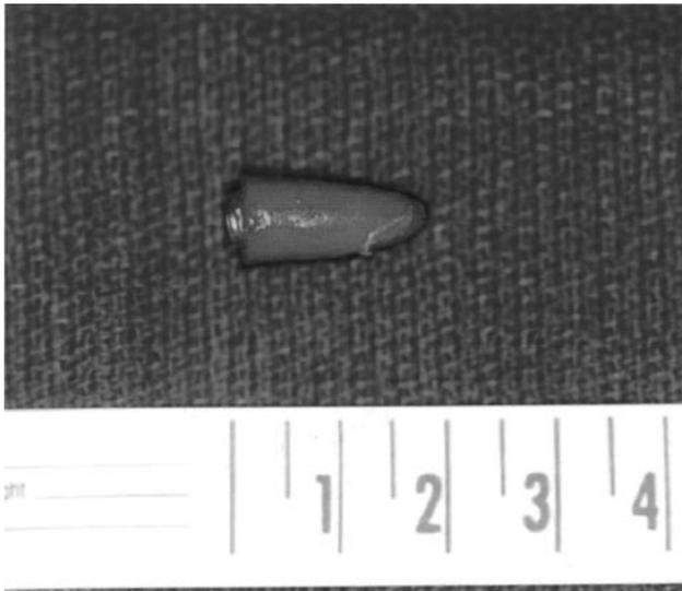
Fig 1. Plastic electrical cap retrieved from the EAC.
