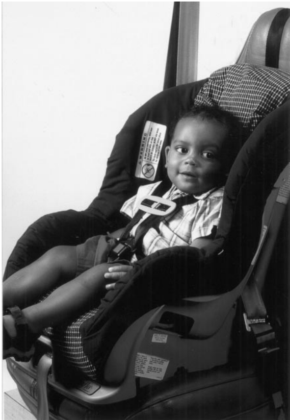
Fig 1. Child safety seat with 5-point harness. Children should be restrained in FFCSSs only when they are at least 1 year of age and weigh >20 lb. FFCSSs should then be used to restrain children until they outgrow the manufacturer's weight limit for the seat.
