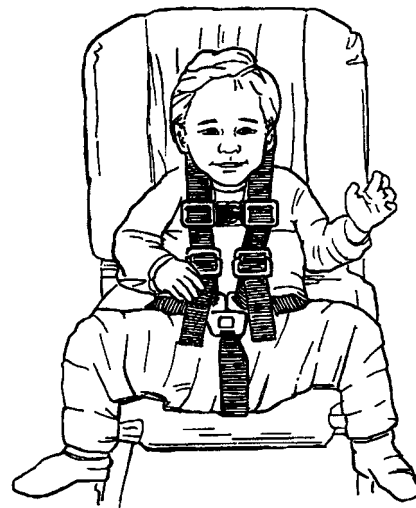
Fig 4. Child with spica cast seated in modified seat with cut-away sides and seat bottom.
