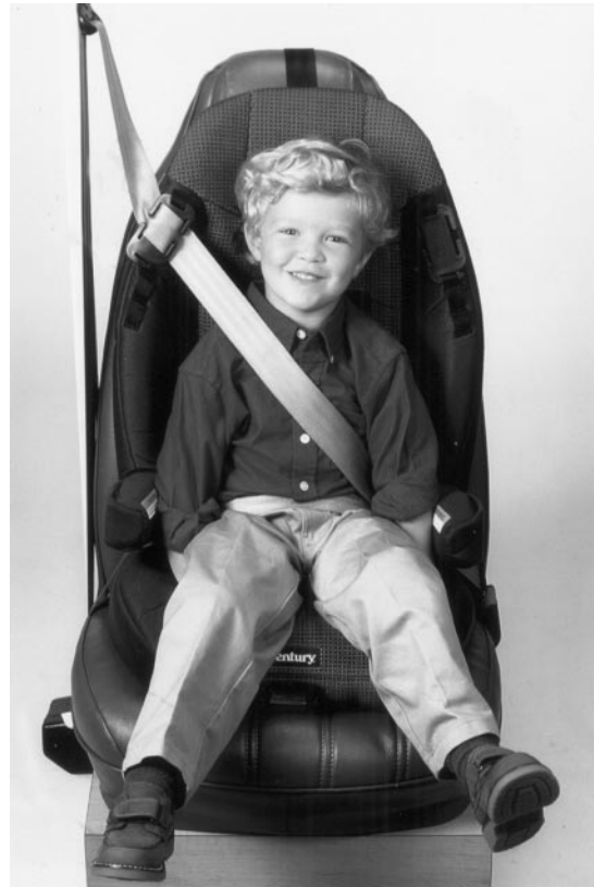
Fig 3. Belt-positioning booster seat. Belt-positioning booster seats should be used in conjunction with the vehicle's 3-point lap and shoulder belt to restrain children who are >40 lb and have outgrown FFCSSs. Belt-positioning booster seats should be used until the child is tall enough for the vehicle's 3-point lap and shoulder belt to fit correctly, usually at ~57 inches in height.
